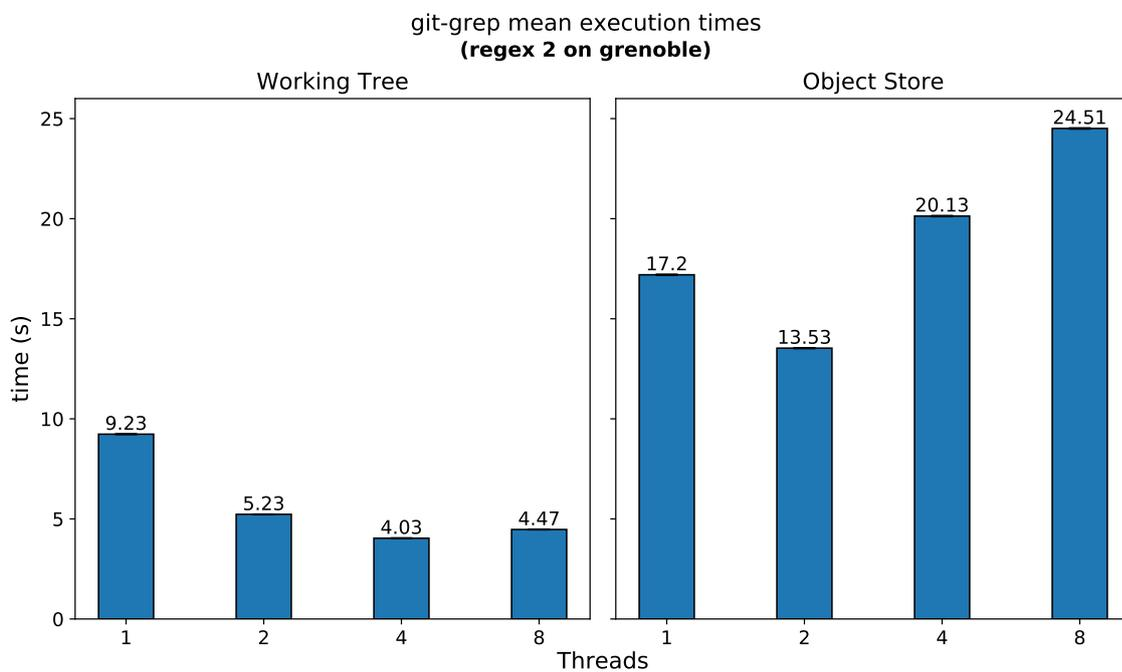
**Figure 1.2:** Mean elapsed time of 30 git grep executions in chromium's repository with regex 2 ("(static|extern) (int|double) \\*"), for different parameters. Executed on machine grenoble (see Appendix A).
