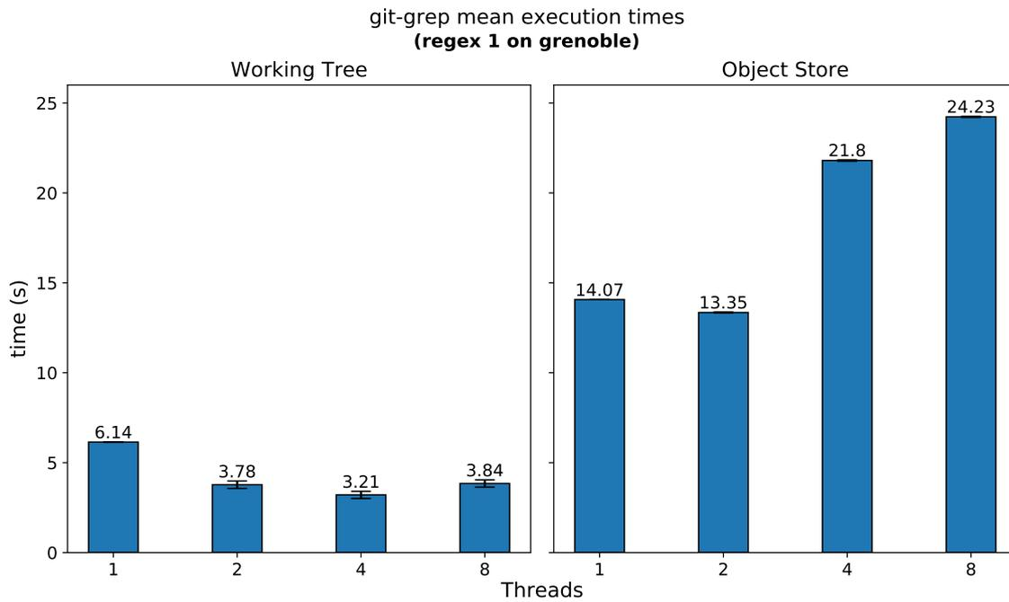
**Figure 1.1:** Mean elapsed time of 30 git grep executions in chromium's repository with regex 1 ("abcd[02]"), for different parameters. Executed on machine grenoble (see Appendix A).
