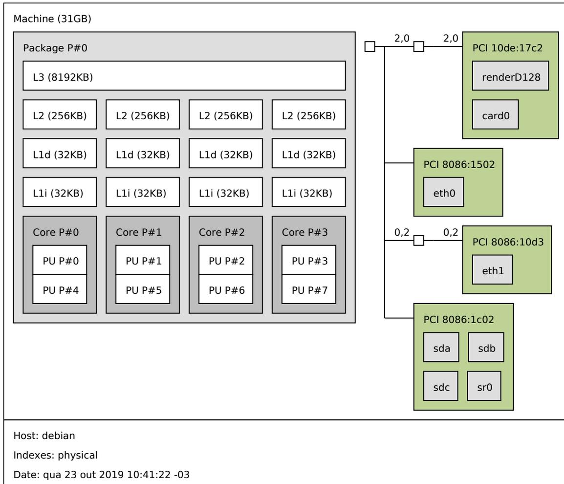
**Figure A.2:** Topology of the machine grenoble.
