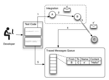
Figure 4.2: Integration test flow example
